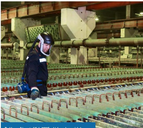
Tankhouse 2 is part of Kola MMC, which produces nickel cathodes using electrowinning technology.
